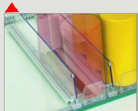
3 The lower fixing cams form a stable compartment when locking with the guide and stabilizer profile, specifically dividers (e.g. for round products on gravity shelves).
